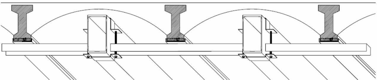
DETALLE MONTAJE DE VIGAS PARALELAS
